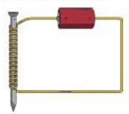
The strength of an electromagnet can be changed by changing the number of coils of wire around the iron core. This can be measured by counting the number of paperclips that become attracted to the electromagnet. Independent variable – number of coils of wire
